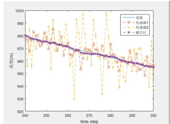
**Fig. 3 Height of track fusion from one flight simulation**
