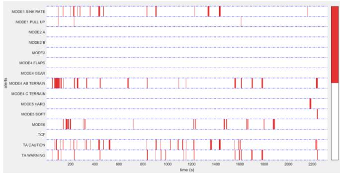
**Fig. 7 Alerts with true trajectory in a single flight simulation**
