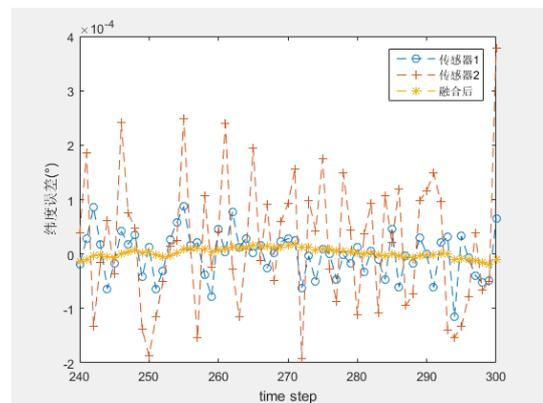
**Fig. 5 Error of latitude from one flight simulation**
