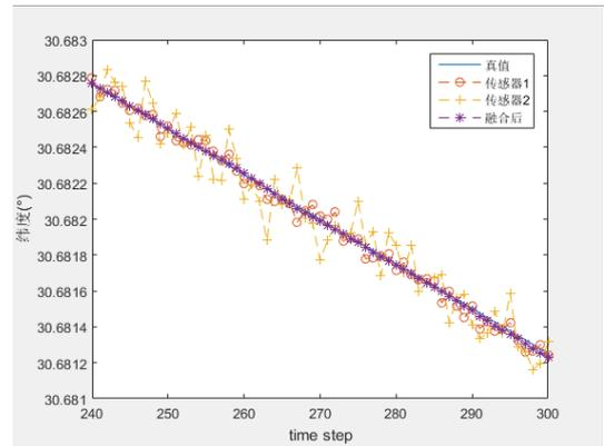
**Fig. 2 Latitude of track fusion from one flight simulation**
