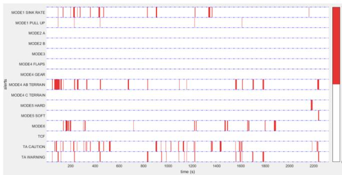
**Fig. 8 Alerts with fused trajectory in a single flight simulation**
